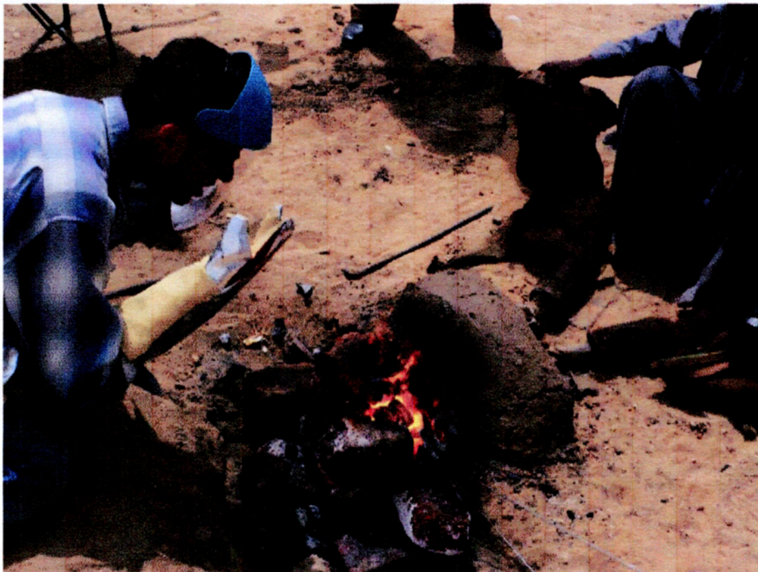
(Blacksmith at work): The melting temperature of bronze achieved inside a small crucible. Blacksmith Kamal Shawki pumps the bellows, archaeo-metallurgist Mark Eccleston watches the result.
