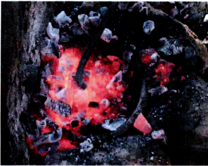
(Red crucible): Air from the bellows' nozzle raises the temperature of the charcoal over the small area of the crucible.
